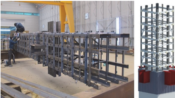
Fig. 1. Encased composite column with steel angles
